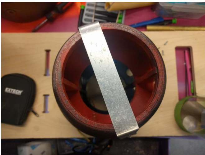
Figure 4 Hole for the pressure tube. Bar over to keep the tube in the squid.
